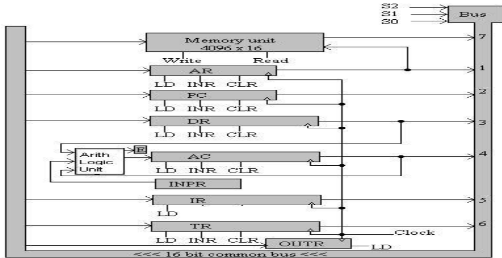
Figure I. The Common Bus System
